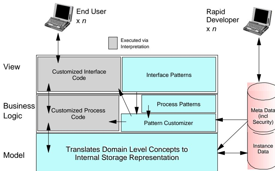
Figure 1 - PAMELA system architecture pattern
